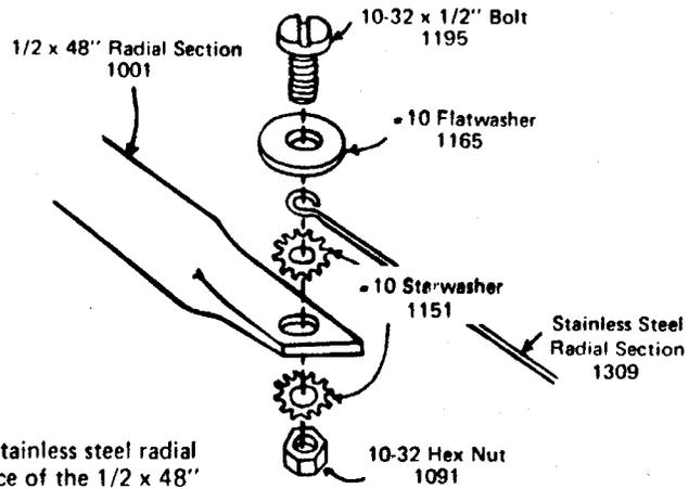
**NOTE:** Use a starwasher between the stainless steel radial section and the flattened surface of the 1/2 x 48" radial section. Use another starwasher between the flattened end of the 1/2 x 48" radial section and the hex nut.
